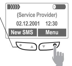
To call up a function displayed, press the soft key underneath the function on the outside.
